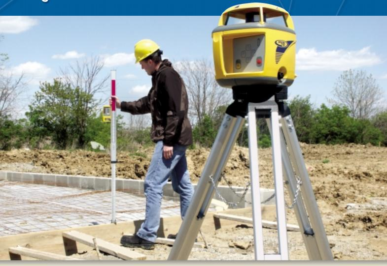
Rugged, reliable and accurate, the Spectra Precision™ Laser LL600 from Trimble sends a continuous, self-leveled 360-degree laser reference over a large work area. This automatic, self-leveling laser is easy to set up and use, and can be used up to a diameter range of 800 meters (2,600 feet).
