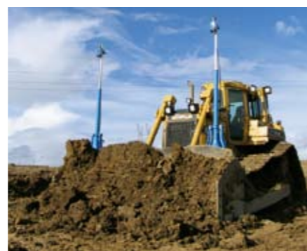
Machine control for dozers, graders, excavators etc.
